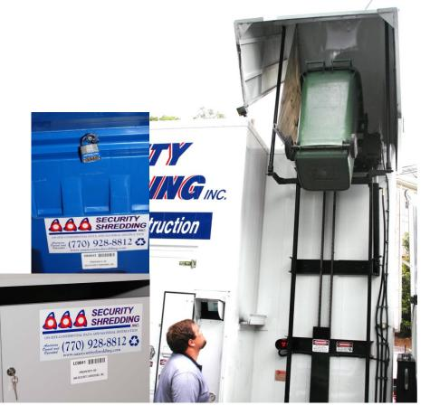
Once outside at the truck, the lock is removed, the materials are automatically fed into the shredder, and are destroyed within minutes. For your peace of mind and privacy, the automated procedure is hands free.
